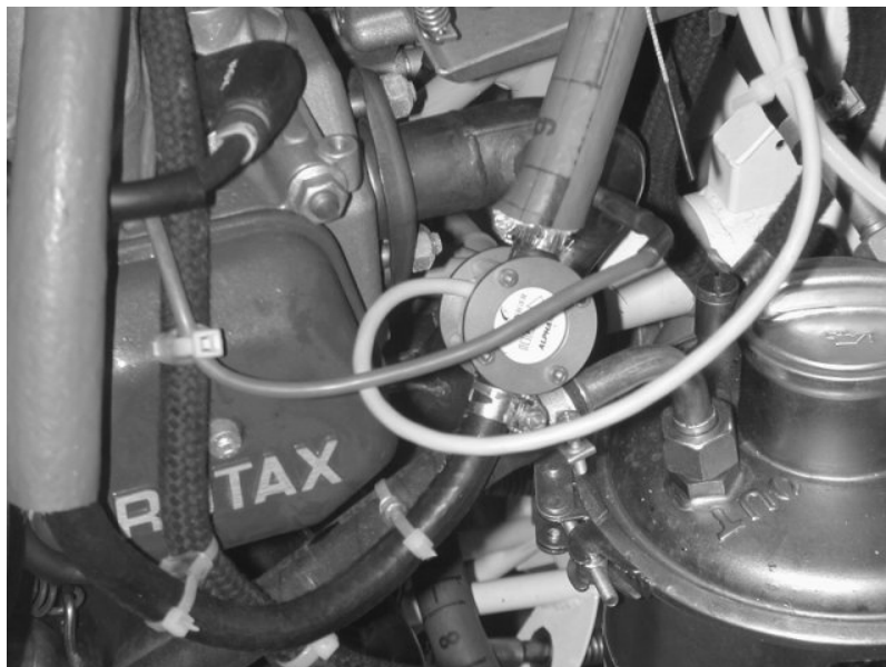
Fuel Flow Sender Mounted on Rotax 912 S as described in Section 5.3.6
